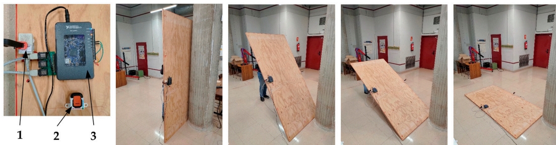
Figure 4. Tilting testing: dual instrumentation and lab set-up. (1) Vibration sensor, (2) inclinometer and (3) myRIO device.
