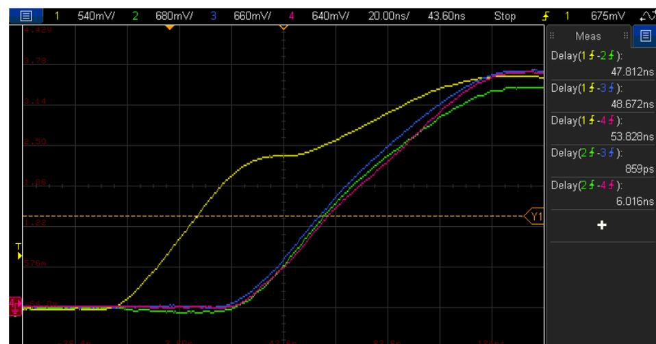
**Figure 3.** Global sync clock (yellow) and sampling clocks of Master Back-end units (green) and two Slave Back-end units (blue and red).
