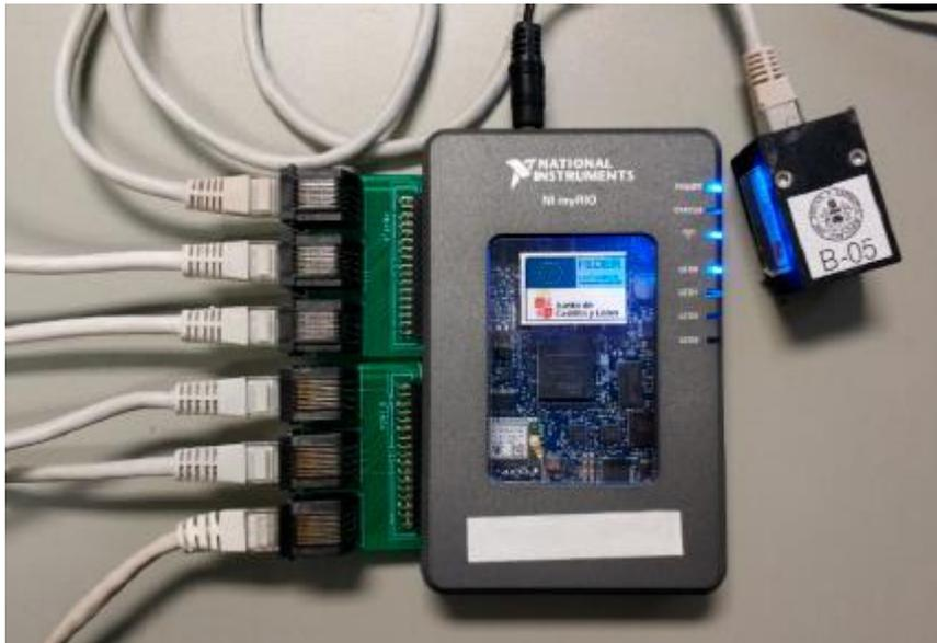
**Figure 3.** MyRIO device with two adapter boards and an accelerometer.
