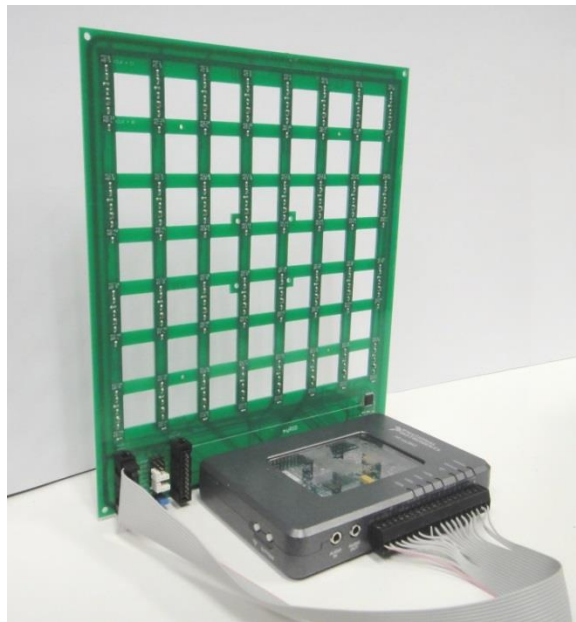
Figure 1. Array module with myRIO and MEMS array board.
