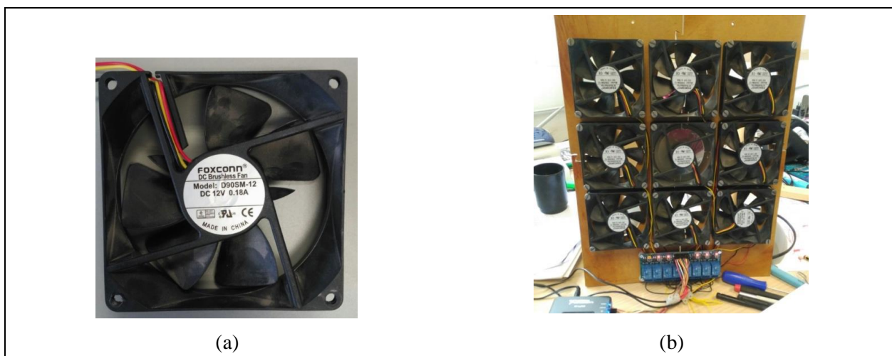
Figure 3. (a) Foxconn D90SM- 12 fan. (b) Fan matrix built for the test.
