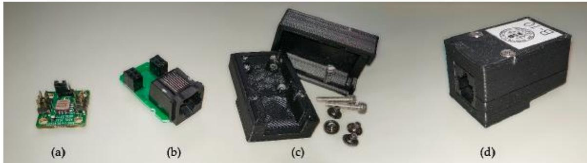
Figure 2. (a) ADXL355 accelerometer (b) adaptor board (c) 3D printed box (d) sensor assembled.
